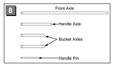
• Identify the front axle, handle axle, bucket axles, and handle pin.
